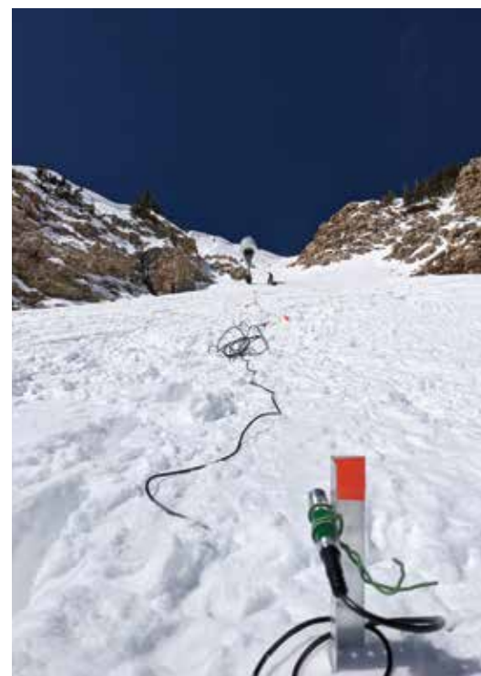
Pressure sensors for testing an O'Belx device at Alta Ski Area.
