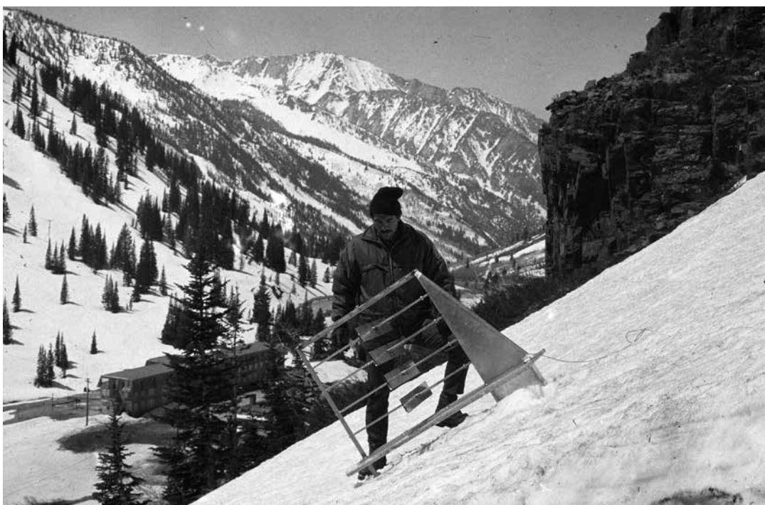
Ron Perla at a creep gage ready to be covered with snow on a test slope next to the Alta Avalanche Study Center. The gage was built by U of Utah, Geophysics (Prof. Bob Smith and team.)
