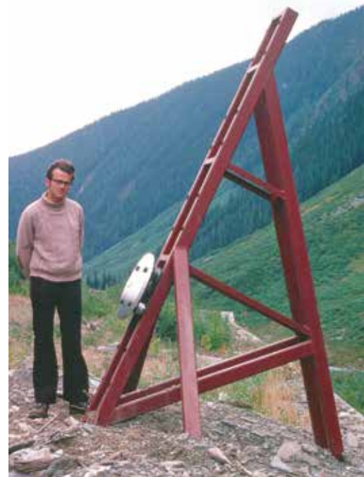
Upslope of a highway shed at Rogers Pass. Terry next to our impact plate mounted on a steel stand installed earlier by Peter Schaerer and Paul Anhorn for their pressure measurements using small pressure cells. ■ RON PERLA, 1978
